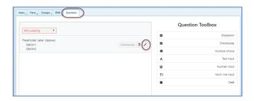
The Checkboxes Editor form will be displayed. In the Label field, type in the name of the Question. If a selection is required by the user, check the Required checkbox. Under Options, two fields are displayed – Option 1 and Option 2. Over type each one with one of the responses to the question. If you have more than two checkbox labels, click the Add Option button to enter another checkbox selection. When finished, click the Save button at the lower right.
